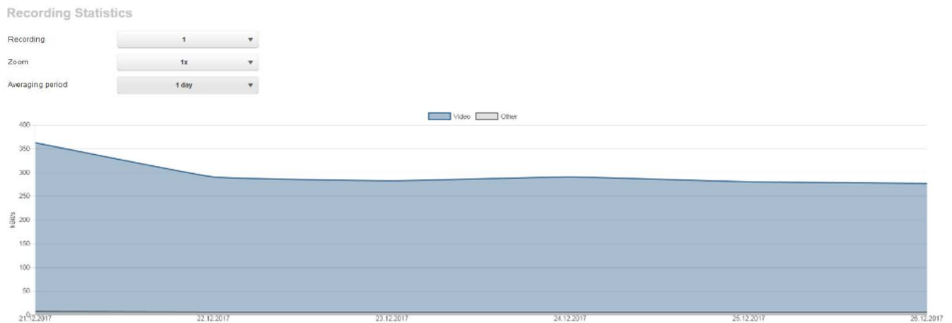
Figure 13: Bitrates with an averaging period of a day captured with DINION IP 4000i IR and H.265
