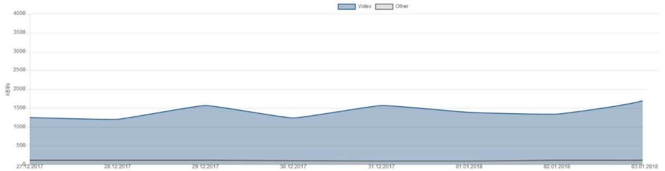
Figure 11: Bitrates with an averaging period of a day captured with DINION IP starlight 7000 HD
