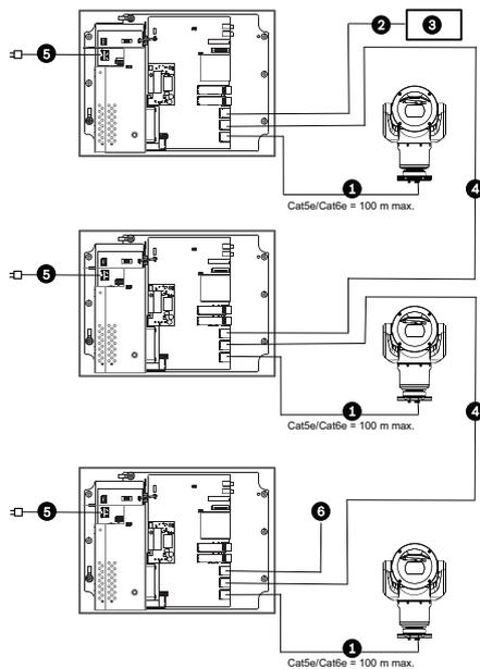
Figure 3.2: Typical daisy chain configuration for VIDEOJET connect 7000
