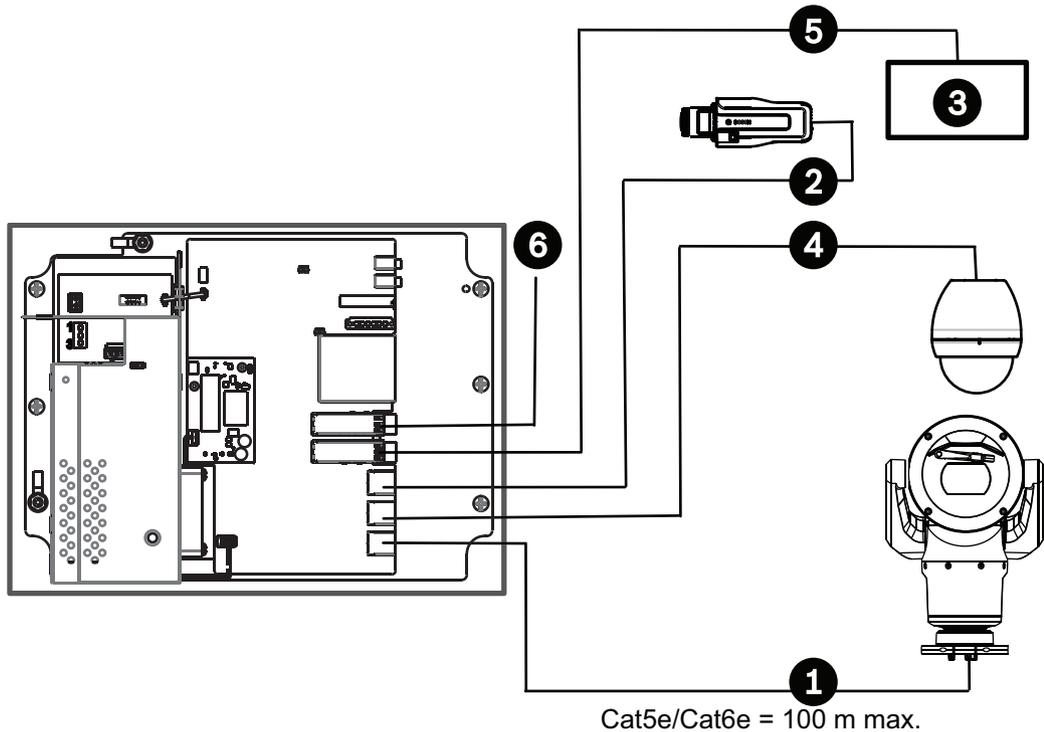
**Figure 3.3: Multiple cameras to VIDEOJET connect 7000**
