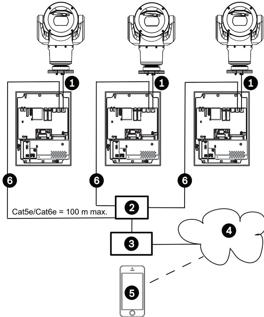
Figure 3.4: Mobile Viewing using the integrated Transcoder of VIDEOJET connect 7000
