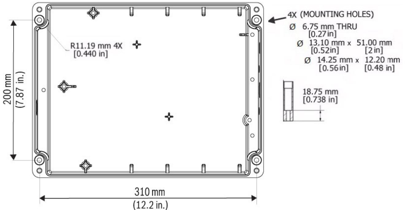
Figure 5.1: Dimensions, mounting holes, VIDEOJET connect 7000
