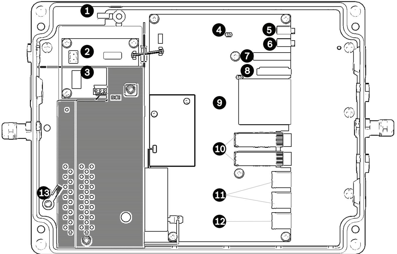
Figure 5.3: Layout of VIDEOJET connect 7000 PCBA
