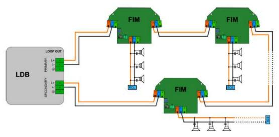
Figure 5.4: T-Branch lines with multiple loudspeakers
