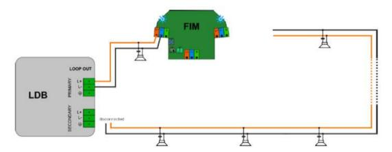
Figure 4.5: Side A of FIM connected to PRIMARY side of the loop
