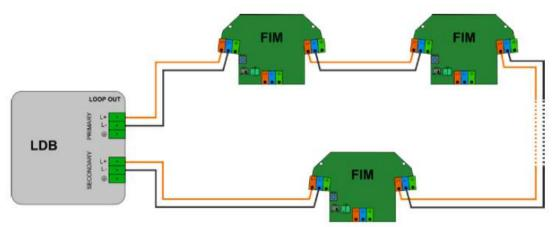
Figure 4.9: Complete loudspeaker line isolator system installation diagram
