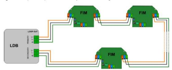
Figure 4.10: Complete loudspeaker line isolator system installation - with optional GROUND wire loop
