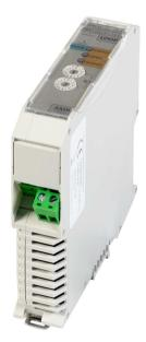
LDB (LoopDrive Booster), with ordering number PRA-LID - is the central unit installed in the Voice Alarm System rack, directly between the amplifier and loudspeaker line. Mounted on a DIN-rail LDB works as the DC-power supply for FIMs and can also generate special service commands to FIMs.
