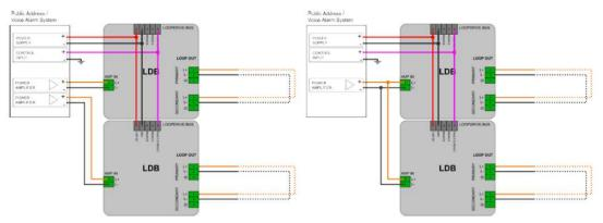
Figure 4.2: Multiple LDB wiring. Left: individual amplifier channels. Right: shared amplifier
