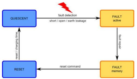
Figure 3.2: Typical loudspeaker line isolator duty cycle
