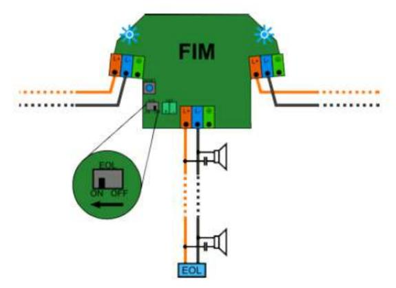
Figure 4.8: T-Branch line with EOL monitoring
