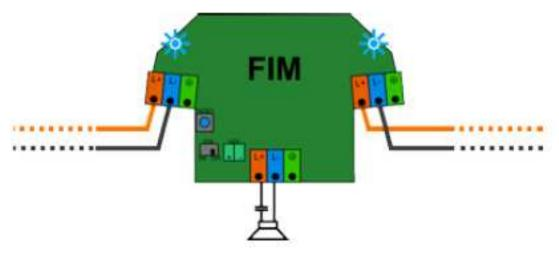
Figure 4.7: Single loudspeaker connected to T-Branch connector
