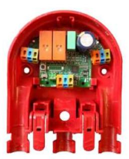
FIM (Fault Isolator Module) with ordering number PRA-LIM - installed in the field, on the loudspeaker line. FIM functions as the isolator in case of a short-circuit. Responsible for monitoring and reporting faults locally (for local line segments connected to the FIM):
