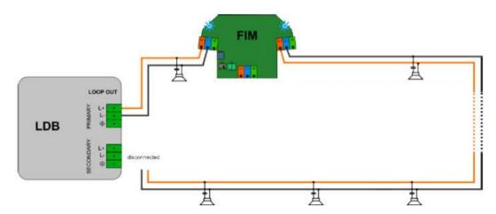
Figure 4.6: Both sides of FIM properly connected to the loop
