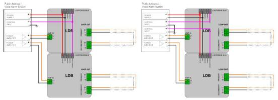
Figure 4.3: Multiple LDB wiring. Left: individual fault contact inputs. Right: common fault contact
