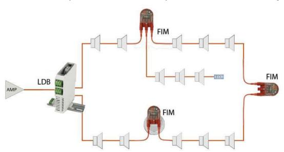
Figure 3.1: Loudspeaker loop monitored by the loudspeaker line isolator
