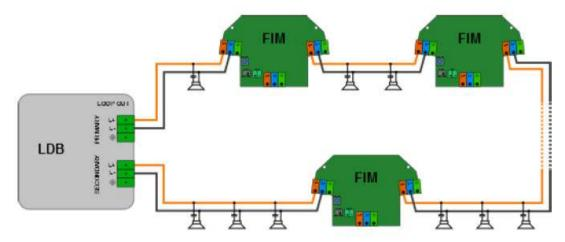
Figure 5.2: Loudspeakers only on the loop
