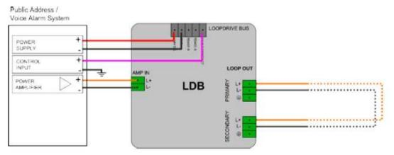
Figure 4.1: Single LDB wiring diagram
