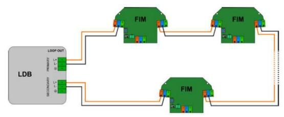
Figure 4.4: Complete loudspeaker line isolator system installation diagram
