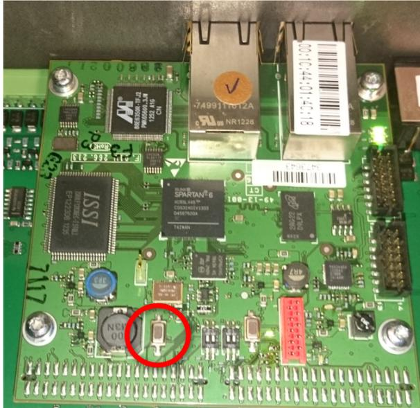
**Figure 7.7:** PRS-4OMI4 PCB non-secure setting
