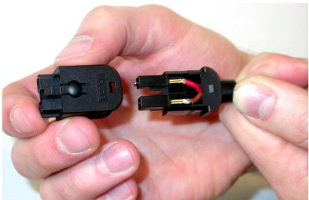
**Figure 6.99:** Mounting the front housing
