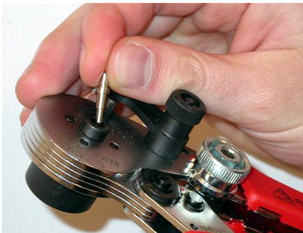
**Figure 6.85:** Inserting a ferrule
