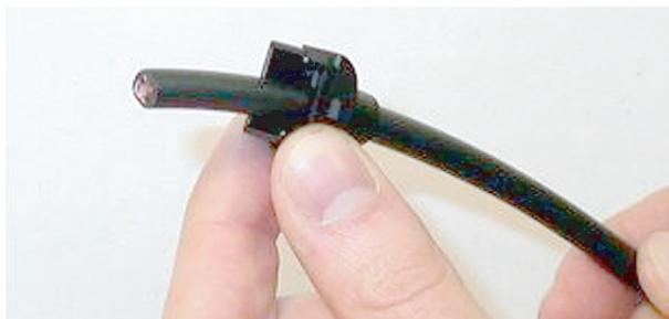
**Figure 6.70:** Back housing on cable
