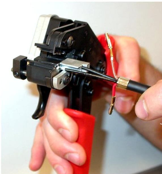
**Figure 6.80:** Cutting a fiber (1)
