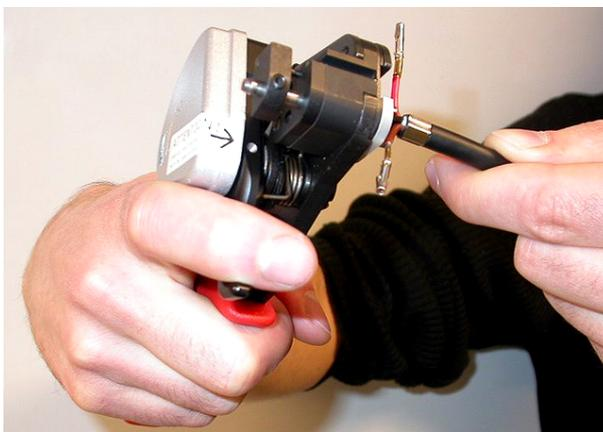
**Figure 6.82:** Cutting a fiber (3)
