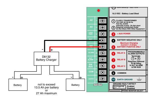
Figure 1: D8132 Battery Charger connection to a 9000 Series Panel
