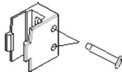
A circuit loop for the strain relief can be wrapped around the plastic clip (mounting bracket) or alternatively around the installation components on the bolt contact ground (see Figure 5).
