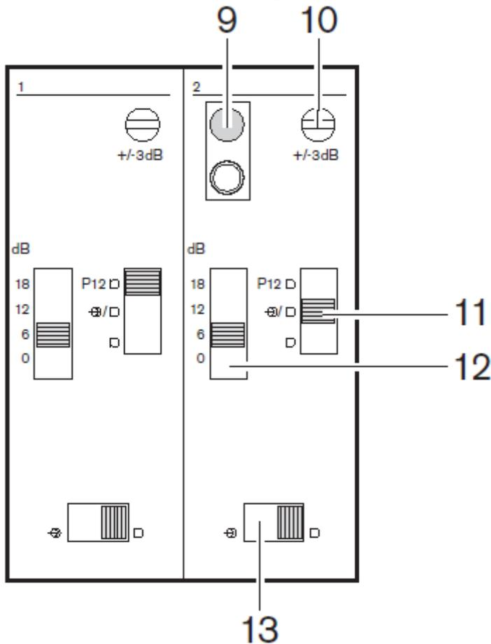
9. De-init switch - Erases the address of the dual delegate interface (refer to Initialization, page 183). The red LED adjacent to the de-init switch comes on when the dual delegate interface does not have an address.
