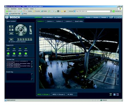
• Launch the Web browser and enter the IP address of the VIP X1600 module as the URL (e.g. http://192.168.0.16) to check that the unit is properly connected to the network.
