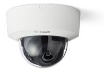
The FLEXIDOME indoor 3100i IR is a versatile camera for general indoor surveillance monitoring. The 5MP sensor, along with an integrated varifocal lens, support a sharp and detailed image with a flexible field of view. With added IR functionality, the camera is able to function even in scenes where ambient lighting is not always available.
