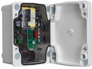
Bosch offers a series of stand-alone power supply units that provide 230 VAC power to AUTODOME 7100i IR cameras for applications without PoE or for redundant power applications with PoE. Each unit has a cover door that provides IP rating IP66/ UL Type 4X ingress protection and meets power and electrical safety requirements in extreme environmental conditions. The unique design and the IK10 rating protect the power supply units from vandalism and tampering events.
