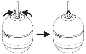
8. Support the **speaker**, snap the support hanger through both main hanger bracket holes located on each individual hanger bracket leg.
