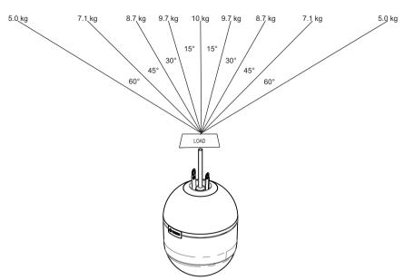
Figure 3.1: Pendant cable working load limit
