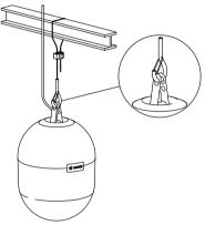
9. Attach a **secondary auxiliary support cable** onto of the secondary auxiliary support hole, located on one bracket hanger leg.
