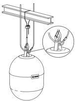
10. Secure the **secondary auxiliary support cable** to a different ceiling support point of the building structure.
