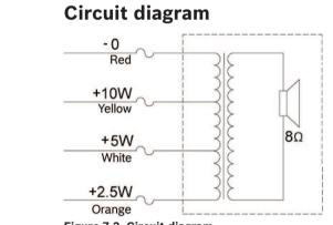
Figure 7.2: Circuit diagram
