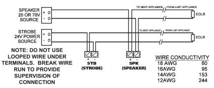
\*MAX. WIRE DISTANCE (IN FEET) = PANEL VOLTAGE - DEVICE MINIMUM VOLTAGE X WIRE CONDUCTIVITY (STROBE ONLY) TOTAL CURRENT DRAW
