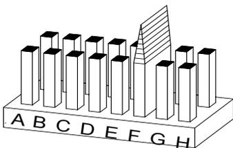
**Figure 4:** Tap Settings (Factory setting is 70V @ 1/2W (Tap F))
