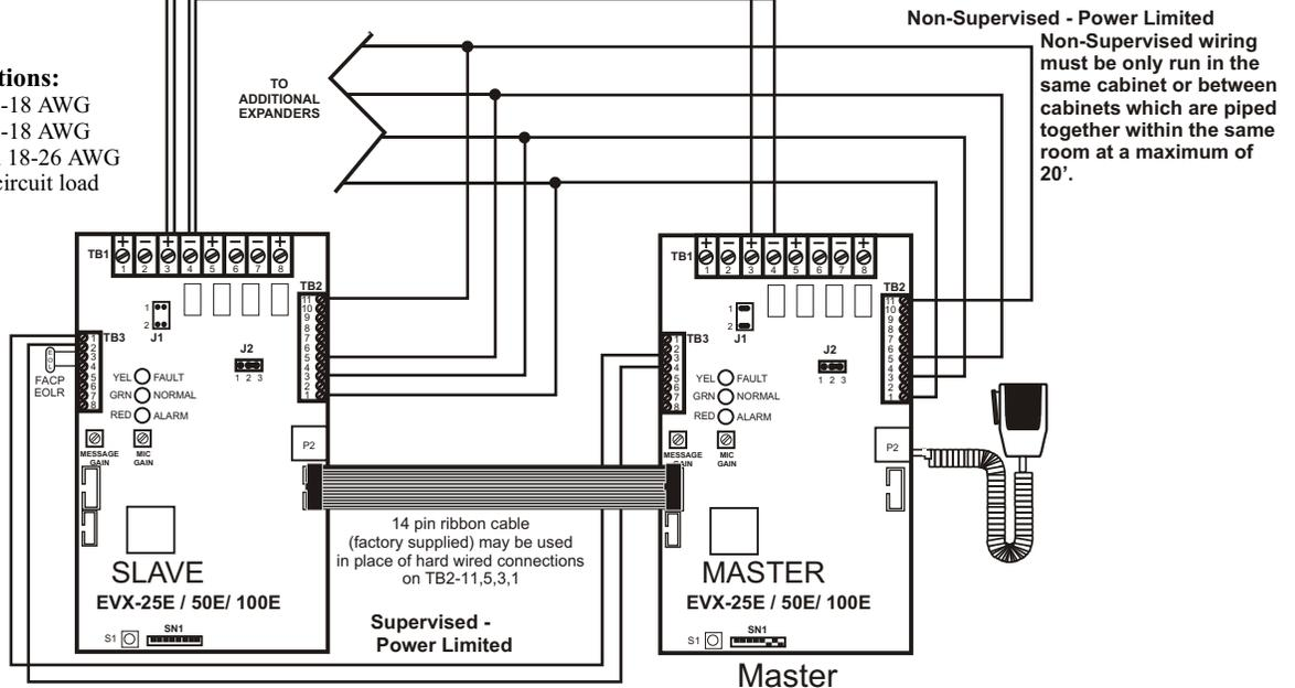
\* NOTE: Switch SN1-6, SN1-8 must be in OFF position for all Slave modules. All Power and Speaker connections remain unchanged.
