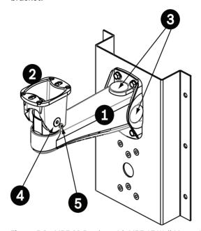
Figure 5.2 MBE-28 Bracket with MBE-17 Wall-Mount Adapter
