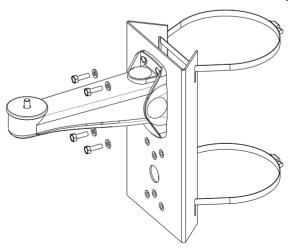
9. Optionally, attach the EXMB.020B to the MBE-15 using the two (2) M6 x 20 hex bolts that shipped with the EXMB.020B. Use the illustration below as a guide:
