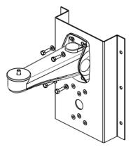
8. Optionally, attach the EXMB.020B to the MBE-17 using the two (2) M6 x 20 hex bolts that shipped with the EXMB.020B. Use the illustration below as a guide:
