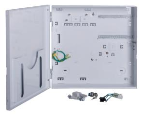
The MAP Expansion Enclosure Kit contains one MAP Expansion Enclosure, one MAP Expansion Enclosure Tamper Switch, one MAP Enclosure Lockset, and one MAP AC Terminal Block. The Expansion Enclosure can house the MAP Power Supply 150W and up to two 18 Ah batteries or four MAP LSN Gateways. It fits in 48 cm (19 in.) mounting.
