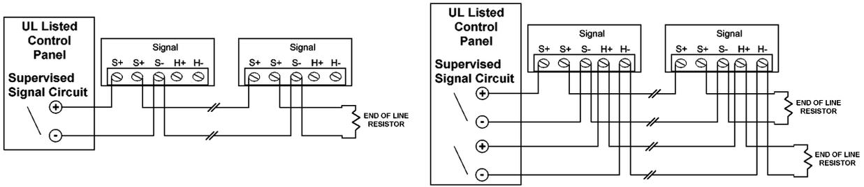
**CAUTION:** When using only a single power source to energize the strobe and horn (switches 1 and 2 up), the in/out wiring must be under the S+ and S- terminals only. Failure to do so may result in damage to your signal. For the horn only (GEH24) and strobe only (WGES), only the top three terminals are to be used.
