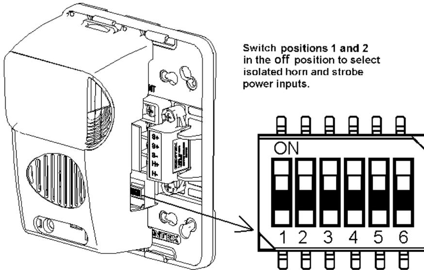
Switch positions 1 and 2 in the Off position to select isolated horn and strobe power inputs.
