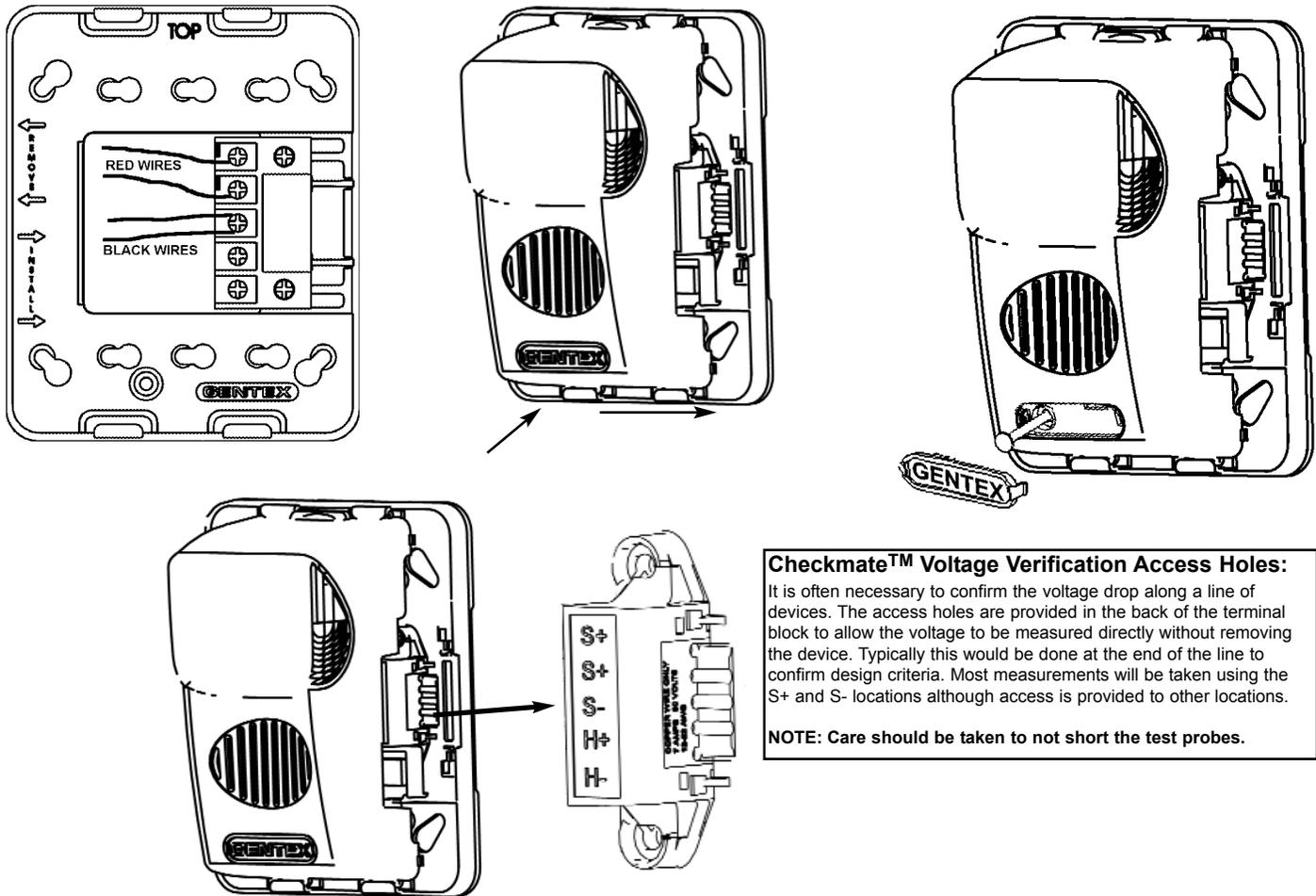
**Checkmate™ Voltage Verification Access Holes:**
