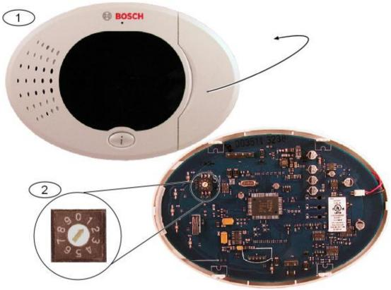
Figure 3.1: Control Center Address Switch
