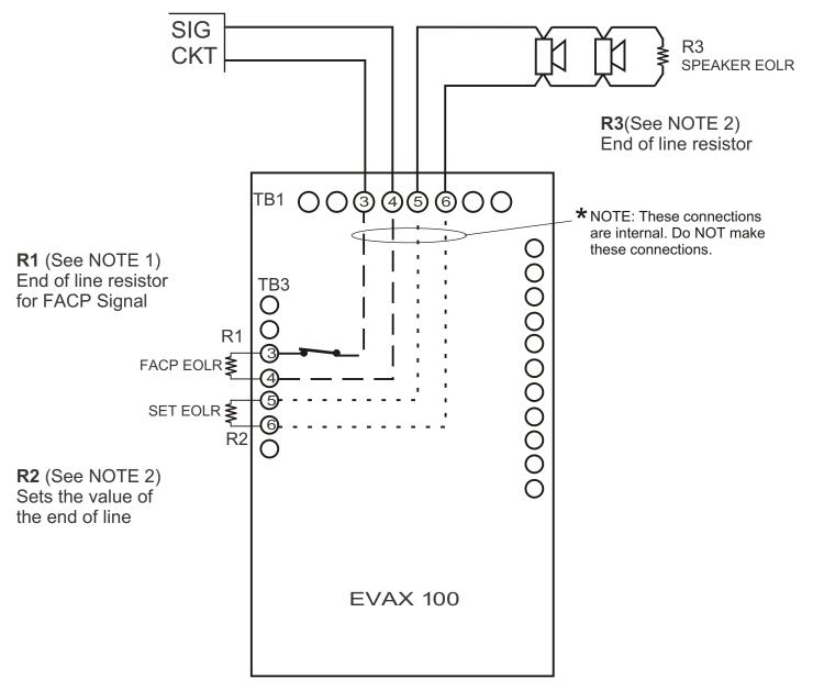
NOTE 1: If the Fire Alarm Signal Circuit requires a 4.7K end-of-line resistor, then R1 must be a 4.7K. Normally, this resistor is connected to the Signal Circuit through a closed Trouble contact. When the EVAX 25/50 goes into Trouble, the contact opens, producing an "Open" on that Signal Circuit,
