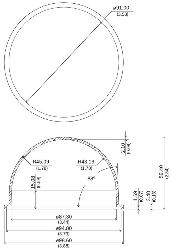
Abmessungen in mm
