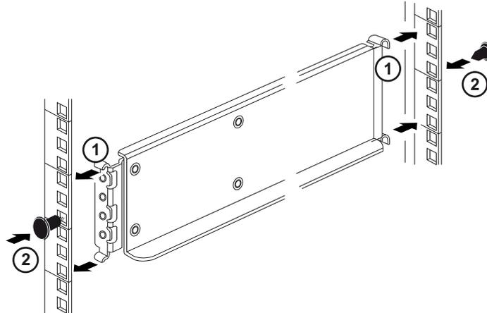
3. Place the back of the unit (the end with the connectors) on the rails.
