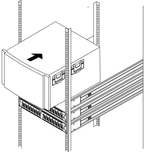
5. Carefully slide the unit all the way onto the rails.
