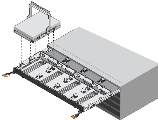
4. Starting with the leftmost slot at the front, align the two raised buttons on the drive with the notches on the drawer. Then, pressing gently on the top of the drive, rotate the drive handle down until the drive snaps into place.
