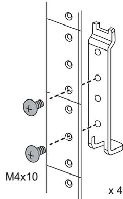
3. Attach the rails to the rack or system cabinet as follows:
