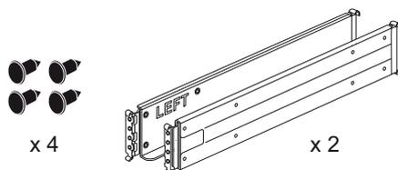
To install SuperRail to square-hole four-post rack:
