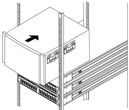
4. Carefully slide the unit all the way onto the rails.
