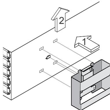
2. Place the back of the unit (the end with the connectors) on the rails.
