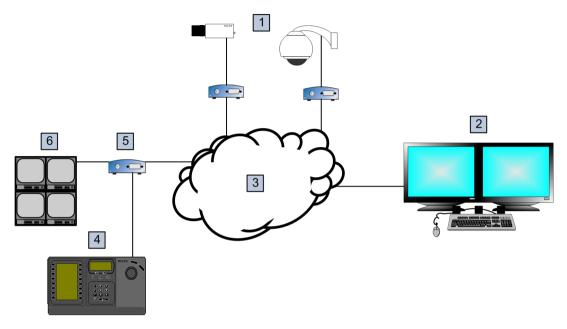
Figure 5.5: Scenario 2: Bosch IntuiKey keyboard connected to a decoder
