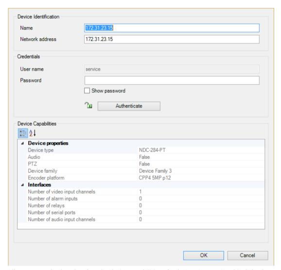
Allows you to check and update the device capabilities of a device. On opening this dialog box the device is connected. The password is checked and the device capabilities of this device are compared with the device capabilities stored in Bosch VMS.
