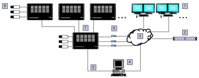
Figure 5.8: Bosch Allegiant system extended with Satellite switches
