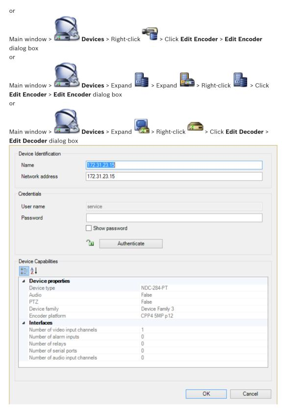
Allows you to check and update the device capabilities of a device. On opening this dialog box the device is connected. The password is checked and the device capabilities of this device are compared with the device capabilities stored in Bosch VMS.
