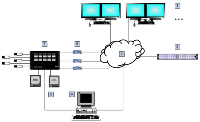
Figure 5.7: Bosch Video Management System remote connection to a Bosch Allegiant matrix switch
