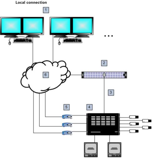
Figure 5.6: Bosch Video Management System local connection to a Bosch Allegiant matrix switch
