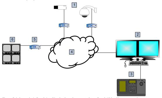
Figure 5.4: Scenario 1: Bosch IntuiKey keyboard connected to a Bosch Video Management System workstation
