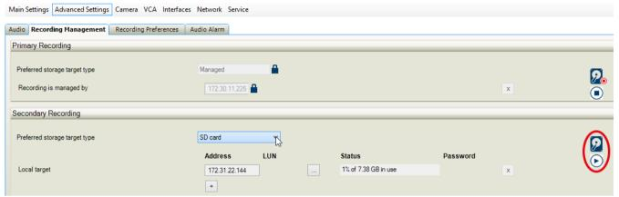
The ANR function only works on encoders with firmware version 5.90 or later. Not all encoder types support ANR even if the correct firmware version is installed.
