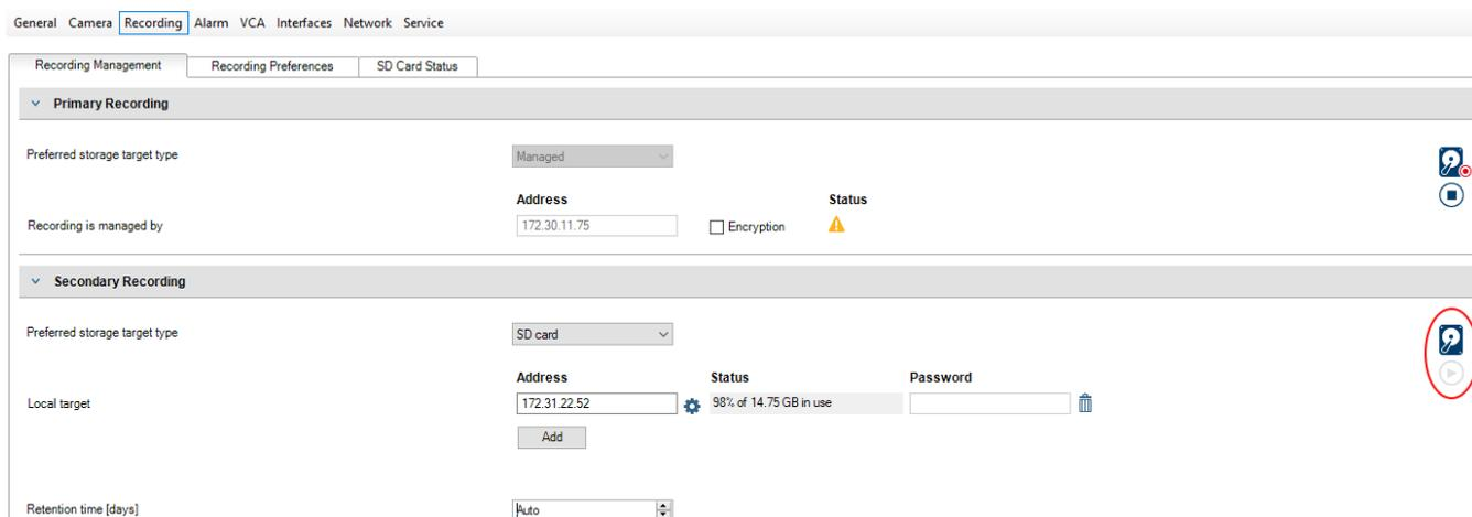
The screenshot shows the 'Recording Management' section of the configuration client. It is divided into 'Primary Recording' and 'Secondary Recording' sections. In the 'Secondary Recording' section, the 'Preferred storage target type' is set to 'SD card'. The 'Local target' is set to '172.31.22.52' with a status of '98% of 14.75 GB in use'. The 'Retention time [days]' is set to 'Auto'. A red circle highlights the 'Info' icon in the top right corner of the 'Secondary Recording' section.
