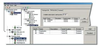
This feature allows the definition and use of the door model "parking lot" which contains the control of two barriers for entrance and exit and their traffic lights, which prevent access when the lot has reached maximum capacity.
