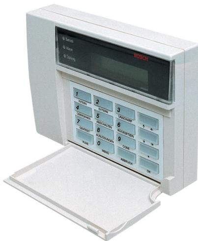
The BE 300 LSN keypad acts as a remote display/control panel for the NZ 300 LSN. The BE 300 LSN is integrated into an LSN loop or LSN stub. Up to eight BE 300 LSN units can be connected. The display/control panel consists of: buzzer to signal alarm, general displays (LEDs) for alarms, faults and operation. Clear text display with 2 lines each of 16 alphanumerical characters (illuminated in event of dialogue) to show all current reports and information. Keyboard operation.
