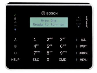
The B921C keypad is an SDI2 bus compatible device. The keypad features capacitive touch keys, instead of the mechanical buttons found on most keypads. With a smooth, sleek surface, the keypad is easy to clean, and fits with any modern decor. The keypad has user adjustable options such as volume and brightness. The keypad has three programmable emergency keys, and four inputs. The keypad also shows two-line system messages for all areas.
