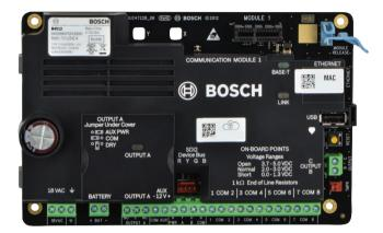
The B4512 Control Panel integrates intrusion and residential fire, providing one simple user interface for both systems. The B4512 provides up to 28 individually identified points that can be split into 2 areas.
