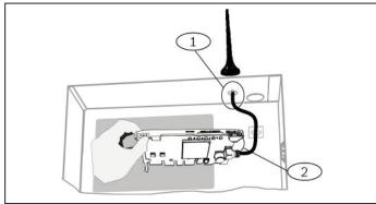
Figure 2.2: Installing the antenna
