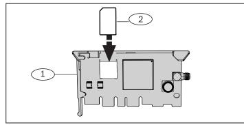
Figure 2.1: Inserting the SIM card
