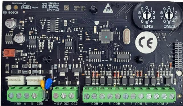
The B228 8-Input, 2-Output Expansion Module is an 8 points/zones supervised expansion device with 2 additional switched outputs that connects to control panels through the SDI2 bus. This module communicates back to the control panel all point status changes, and the outputs are switched on and off through a command from the control panel. The inputs and outputs are accessed through on-board screw terminal connections.
