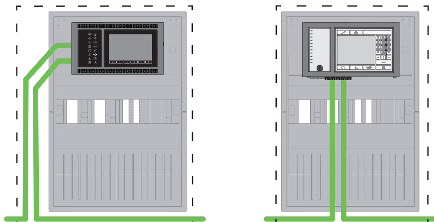
Figure 7.2: Panel network over CAN
