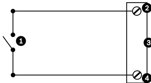
Figure 14.5: N.O. - Normally Open Non-supervised Connections
