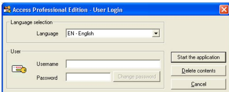
The upper drop-down list can be used to select the desired interaction **language**. The default is that language which was used to install the application. If there is a change of user without restarting the application then the previous language is retained. For this reason it is possible for a dialog box to appear in an undesired language. In order to avoid this, please log in to Access PE again.
