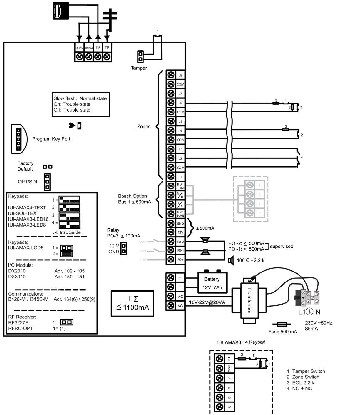
Figure 3.3: Wiring diagram AMAX 2100 / 3000
